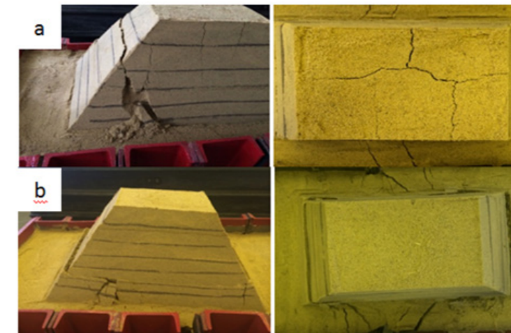
Figure 8 – Comparison of stability modeling key stages for dam model without reinforcement; (b) with reinforcement)
