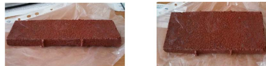
a) – with the proportions of fillers 1:1:1, b) – with the proportions of fillers 1:1,5:0,5 mm
