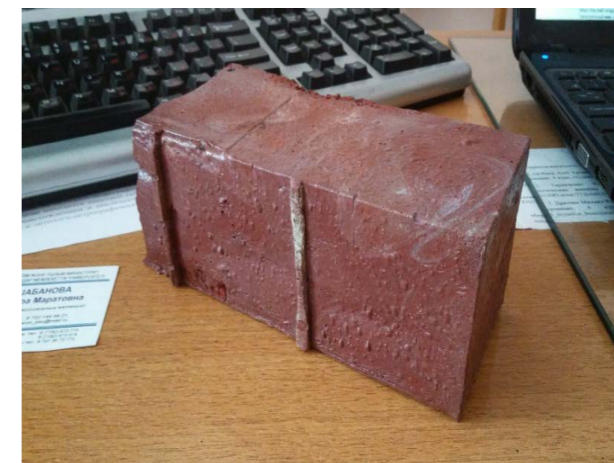
Picture 5 – Models with dye from plastic materials by faction a 2x2x1 mm, with the proportions of fillers 0,5:1:1,5
