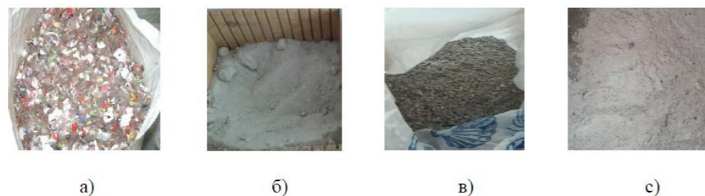
a) – chopped plastic (LDPE), b) – river sand, c) – ash of Ekibastuz coal, d) – aspiration ash of metallurgical production Picture 2 – Used raw materials
