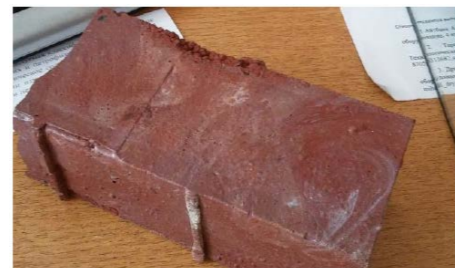
Picture 7 – is a standard from plastic materials by faction 2x2x1 mm, with the proportions of fillers 1:1,5:0,5 and with the use of metallurgical slag
