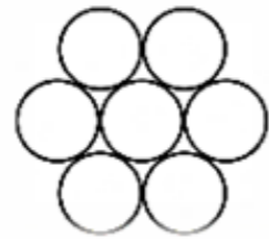
Figure 1. Construction of a seven-wire reinforcement rope 1×7
