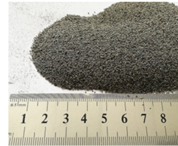
Figure 1 – Fly ash of Pavlodar thermal power plant-1
