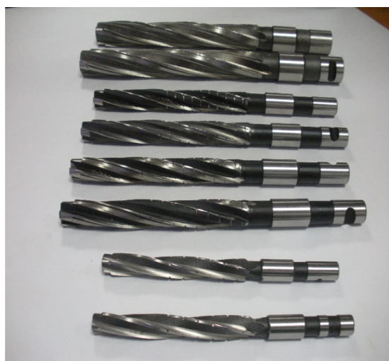
Figure 3 – Prototypes of the sweep-broach
