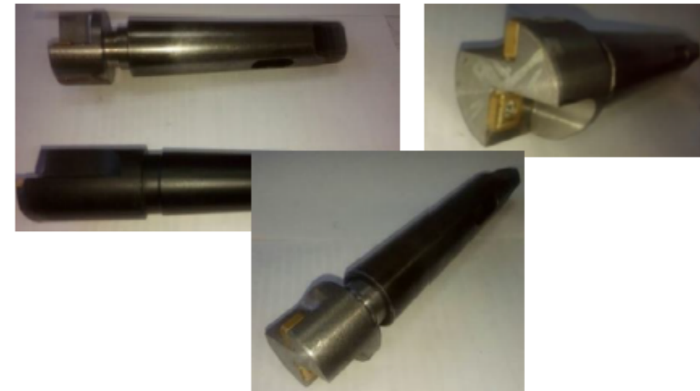
Figure 4 – Prototypes of combined cutting head
