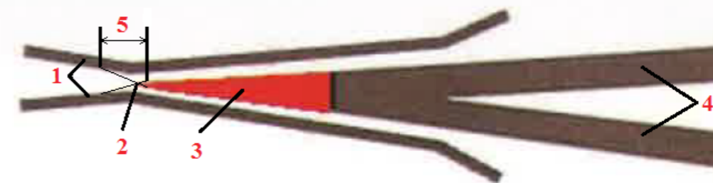
Figure 2 – VAE cross scheme: 1 – kicking rails; 2 – mathematical centre; 3 – core; 4 – crucifixion tail; 5 – harmful expanse [13]
